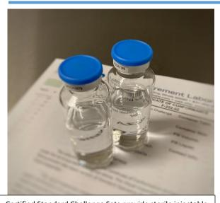
Certified Standard Challenge Sets provide sterile injectable product manufacturers with a durable, precision-manufactured challenge set that can be used to train and qualify inspectors and automated inspection machines. Certified sets means higher confidence in POD data.
